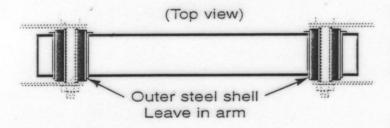
The original equipment am has an outer steel shell into which is pressed the steel shelled bush.
